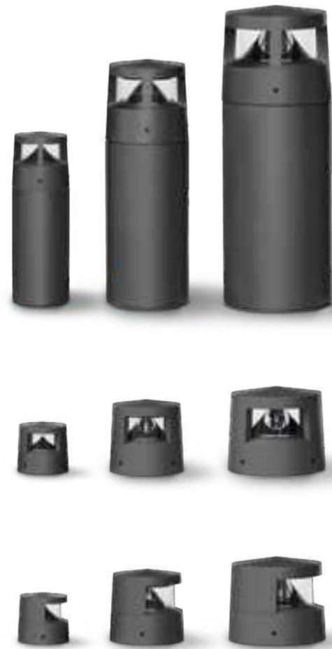
Reef is a range of short bollards with radial lighting emission obtained with a specific conical reflector. Perfect to illuminate with grazing lighting effects walking areas of residential, parks and public spaces, are available in three dimensions. The polycarbonate diffuser ensures a high impact resistance.
