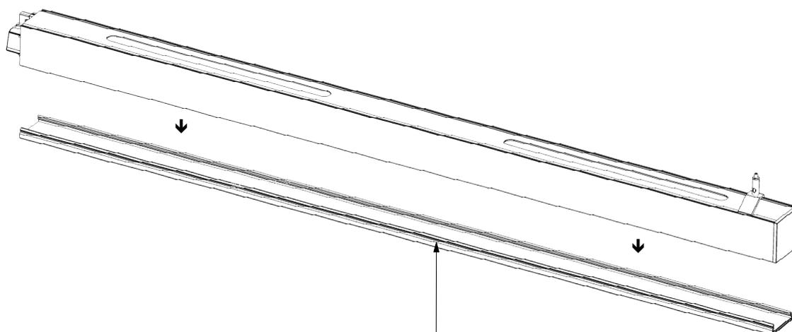
Diffuser/Louvre needs to be removed to gain access to the internal fixing screw to fix modules together.
