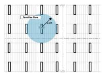
Motion Sensor - Detection Range of a single Sensor Node imposed over a Typical RCP (2.5m circular radius, 2.7m luminaire height.
