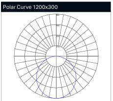
Maximum Candela = 860cd/klm Located At Horizontal Angle = 22.5, Vertical Angle = .5
